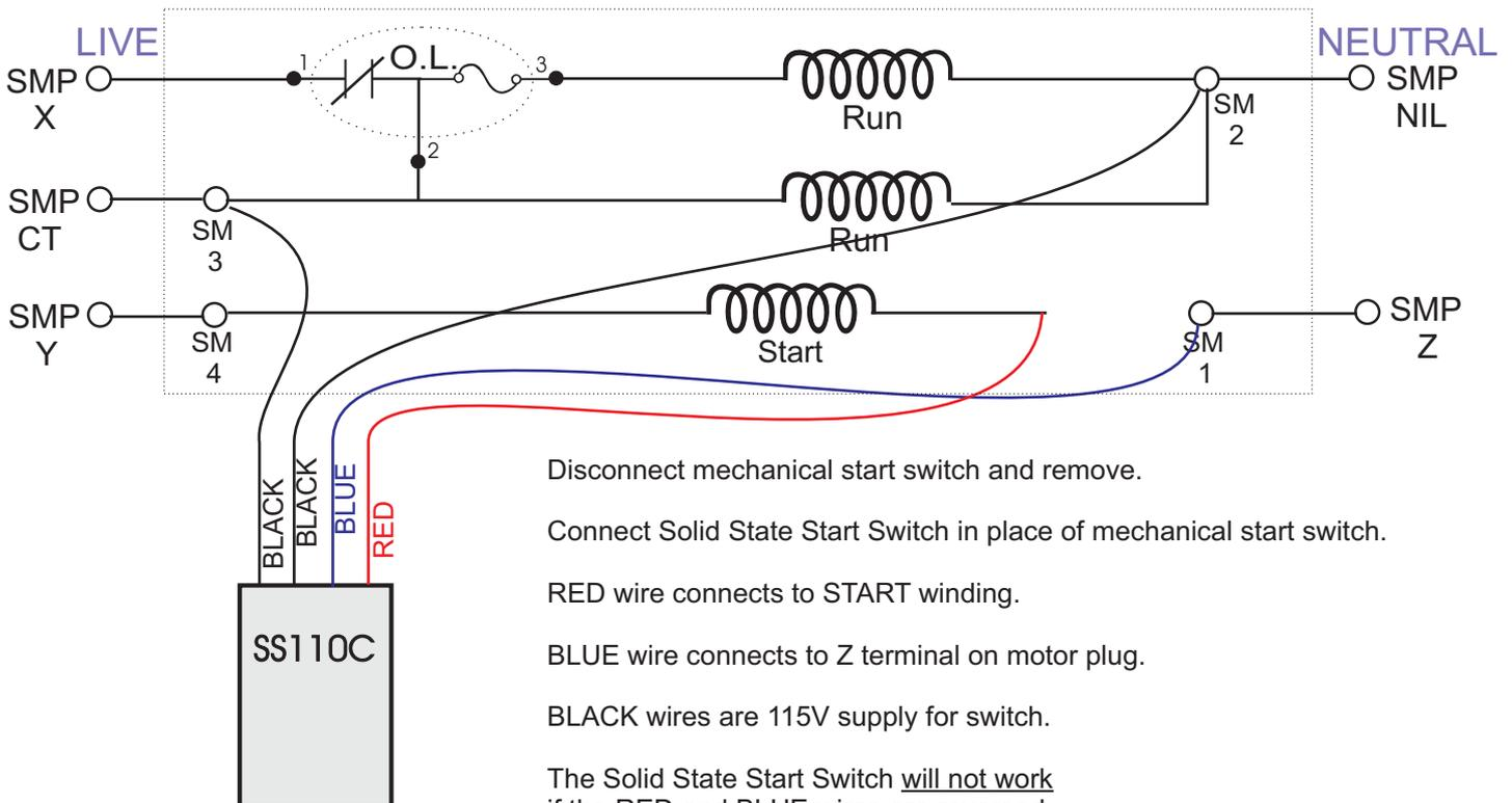
Disconnect mechanical start switch and remove.
